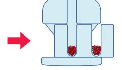
3 In use, the patient pushes the dose compartment sideways and aligns the first dose compartment with the mouthpiece.
