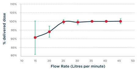
The minimum flow rate at which TwinCaps<sup>®</sup> has been shown to deliver 95% of the nominal dose is 20 litres per minute of airflow. Above 25 litres per minute, performance is unaffected (data formulation dependent).
