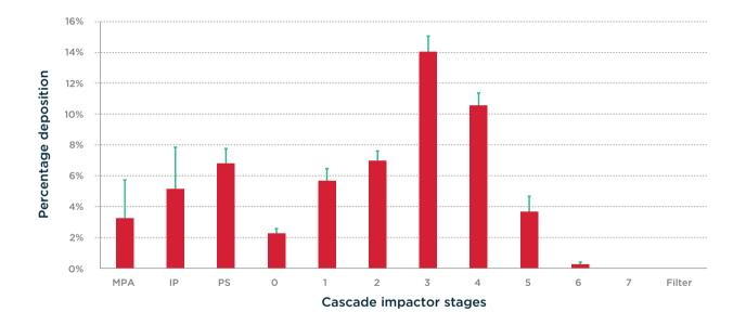
In the NGI test illustrated above, a reproducible, lung delivered dose of 58% was obtained. The percentage of drug deposited in stage 3 and below was 28% in relation to the label claim, and 58% in relation to the emitted dose, possibly implying retained drug in the inhaler is composed of larger particles.
