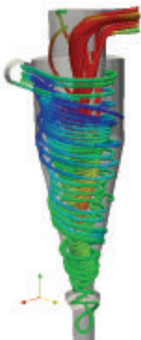
Figure 5: CFD predictions for the flow pattern in a cyclone
