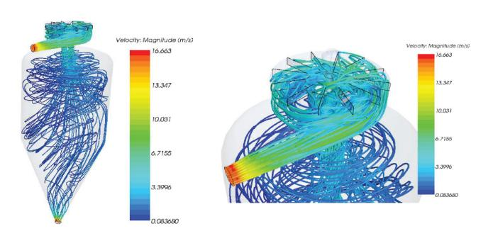
SD1252: Streamlines colored by velocity magnitude at middle plane: full view (left), injection region detail (right, fixed scale)
