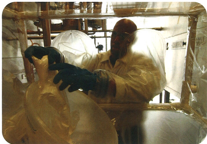
Picture 4: Operator charging reactor using flexible containment during surrogate testing.
