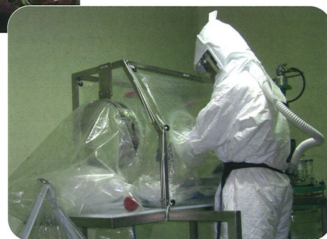
Picture 2: Operator charging reactor using flexible containment during processing.
