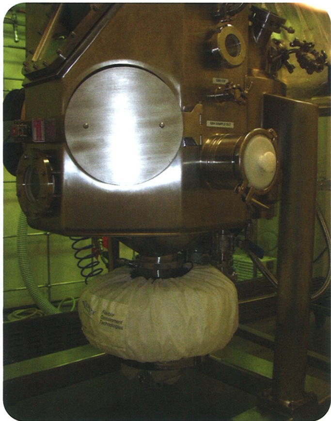
Picture 3: Filter Dryer discharge with continuous liner (flexible containment).
