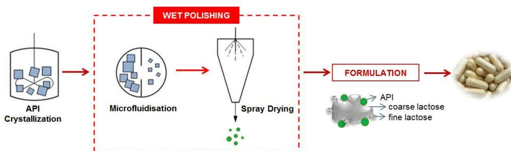
**Figure 1.** Schematic representation of the Wet Polishing (WP) technology.
