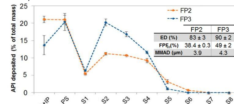
**Figure 4.** NGI aerodynamic deposition of FP2 and FP3 where ED, FPF, MMAD, MPA, IP, PS and S1 stand for emitted dose, fine particle fraction, mass median aerodynamic diameter, mouthpiece adaptor, induction port, pre-separator and stage 1 respectively.
