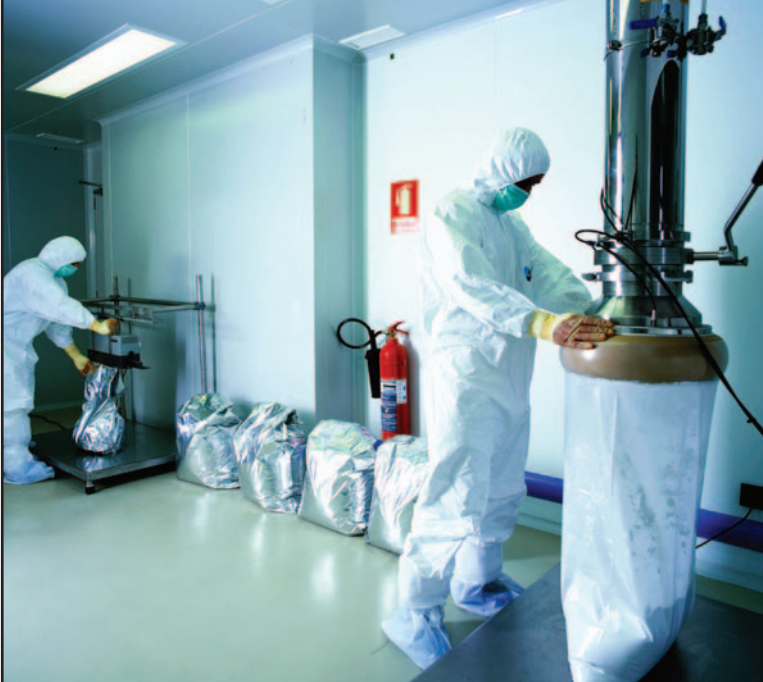
Discharge of final product into a classified clean room.
