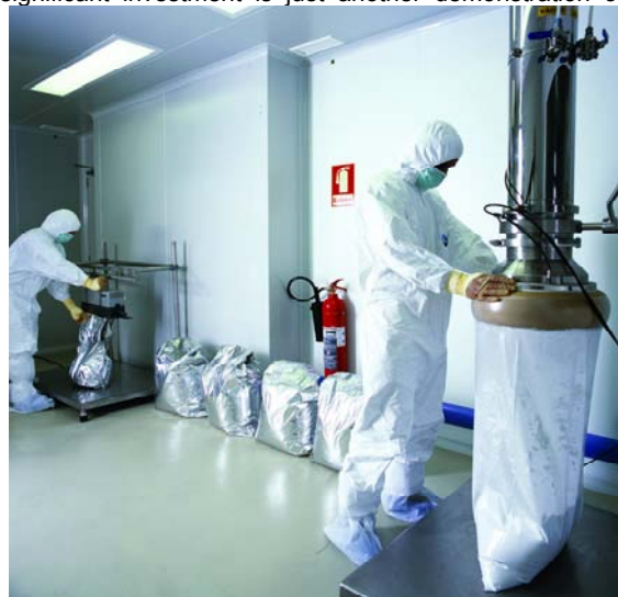
Discharge of final product into a classified clean-room
